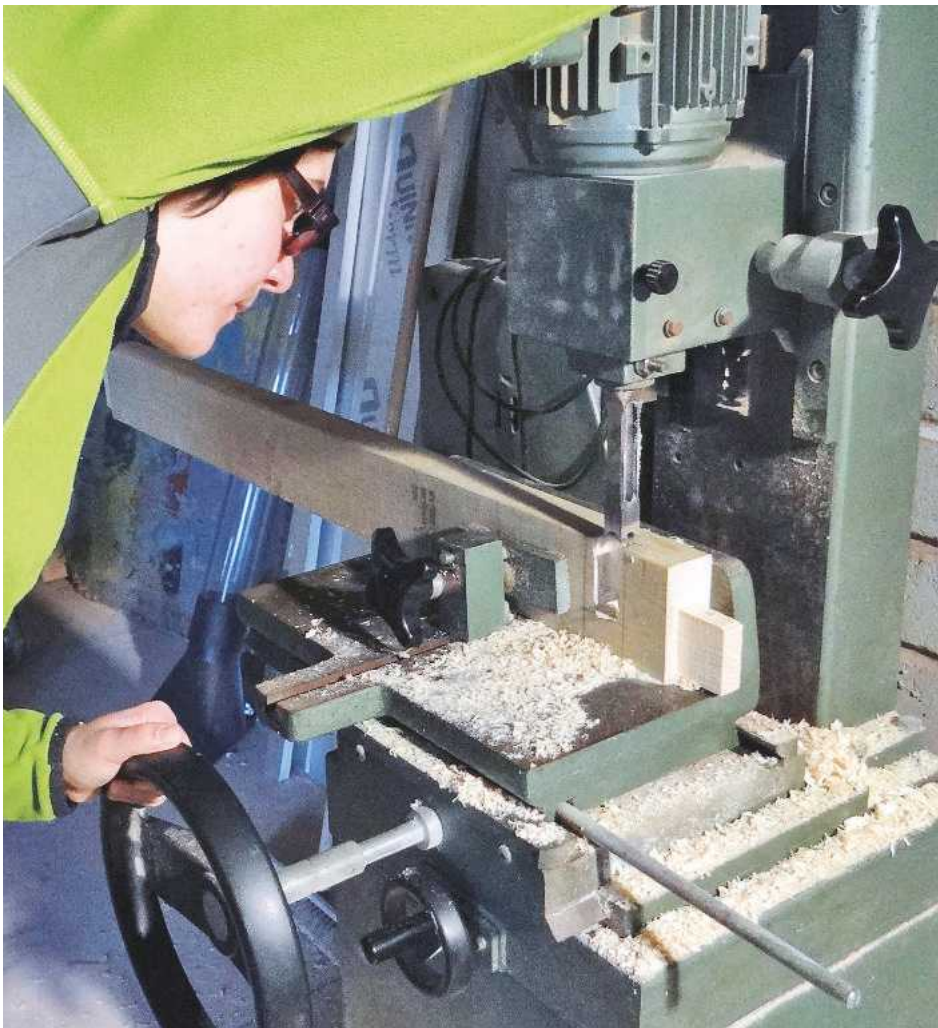
▲ Pic.2 The Swiss watch: precise, dependable and effective. Here Aurelia is using the mortiser to chop out the stopped housings for middle rails. A through mortise and tenon would have been an alternative, but given that all the weight was downwards, I considered this the stronger joint
